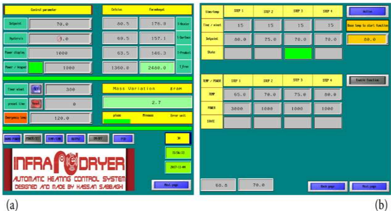
Fig. 2. Different sections designed by ADP software, temperature, power and weight setting and monitoring (a), settings for a stepwise process at different temperatures (b)
