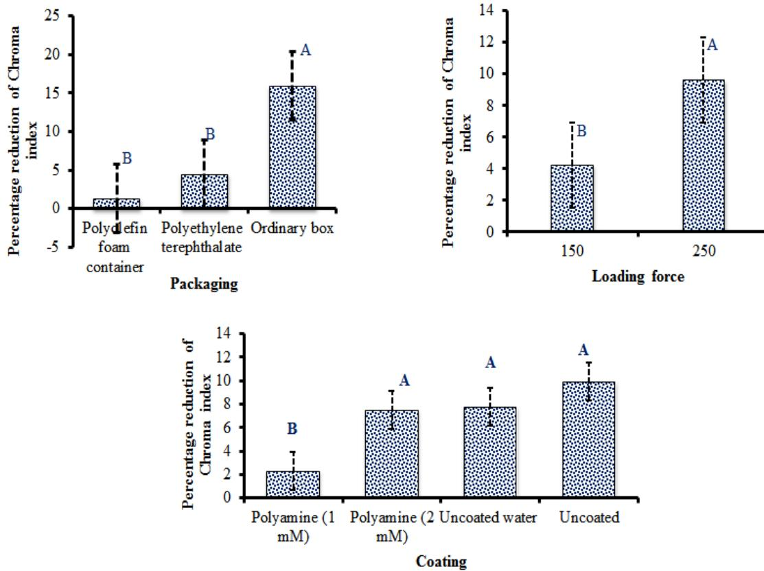
**Fig. 4. Comparison of average on Chroma index value, a) Packaging, b) Loading, c) Coating.**
