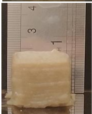
Fig. 4. 3D printability evaluation (cubic) of 3D printed gels prepared with QP (B/CP/PEF) and Ag-SA at 25 °C
