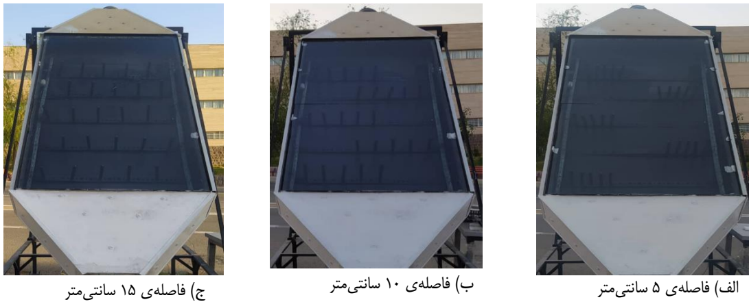
Fig 2. The place of tubes containing phase change materials perpendicular to the absorber plate
