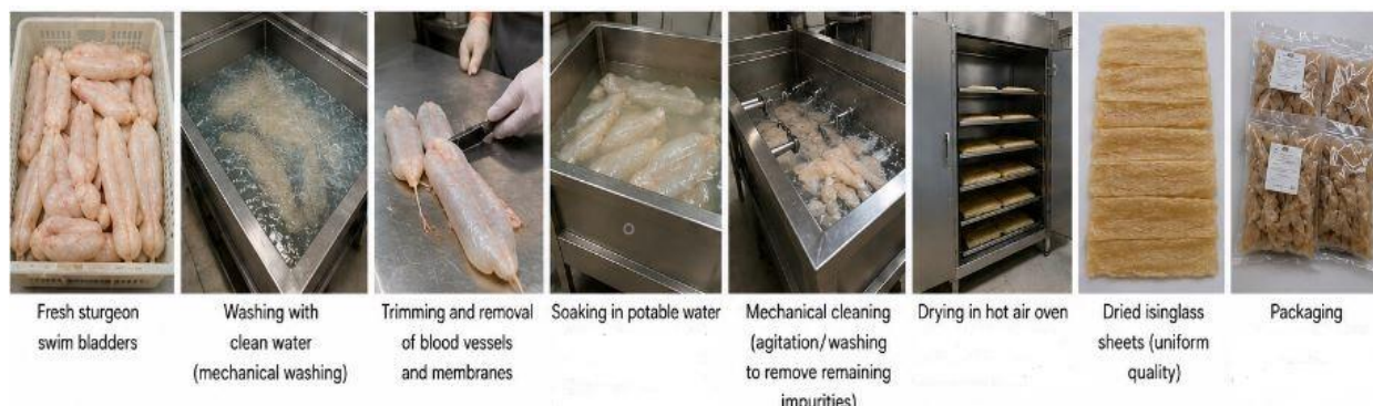
Fig. 2. Preparation of isinglass from sturgeon swim bladders by semi industrial method
